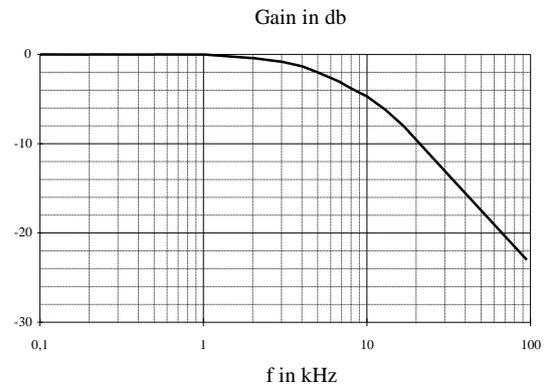
The chart shows dependence of amplitude of the application circuit with OP-amp = AD795,  $R_f = 10 \text{ M}\Omega$  and  $C_f = 1 \text{ pF}$
